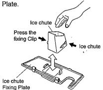
\* Clean Ice Chute with soft cloth or sponge. Shaved ice can be clogged if the inside surface of Ice Chute is scratched.
